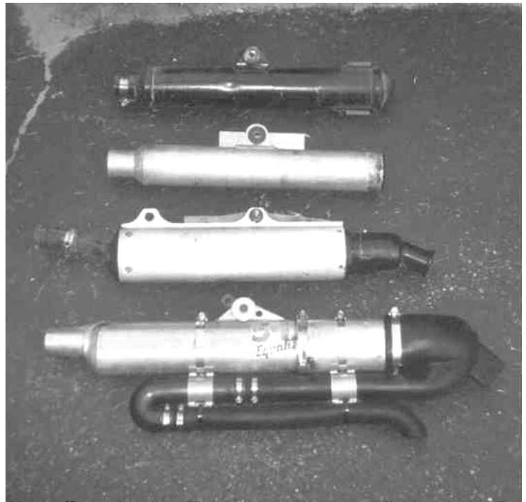
My muffler collection. The only one that beat Michigan's 94dba limit without any noticeable power change was the Answer Equalizer with the dB Snorkle attached.
